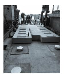
FST on Rubber Bearings: Ningbo Fengshua Line
