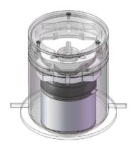
Floating Slab Track (FST) on Steel Springs
